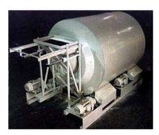
The Inventure High Intensity Drum Mixer discharges simply by reversing the direction of rotation, eliminating a complicated tilting mechanism and hydraulics. The resourceful mixing blade arrangement and the non-tilting drum provides shorter mixing time and energy costs will be reduced.
